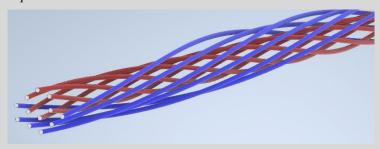
Most multiple conductor cables make use of this trick. Conductors are kept apart with different means. Conductors have to be kept from touching, of course. In machine built cables, various plastic materials are used to fill interconductor space.
