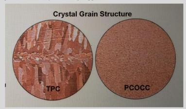
Tough Pitch Copper and Pure Copper Ohno Continuous Cast.
